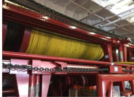
Photograph provided by Total showing Leadon flowline packed onto anchor winch drum.
